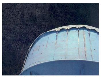
**Figure 4: Missing Radome Mounts**
